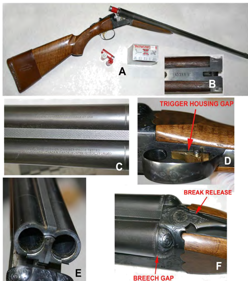
Figure 4: The shotgun. A: Full view of the Ithaca shotgun with the Winchester-ame Load box and cartridges used in the test of the shotgun. B: The serial number of the shotgun. C: Identification information on the barrels of the shotgun. D: The trigger area of the shotgun. The trigger housing gap is indicated. E: The opened breech of the shotgun. F: The closed breech area of the shotgun.
