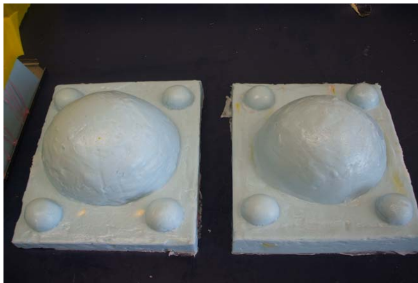
Figure 7.2 The two different sized positive plugs. The larger plug (left) was used to create the “skin” layer, while the smaller plug (right) was used to create the “bone” layer. The orientation plugs, in each corner, correspond to the orientation holes on the negative mould (Figure 7.1).
