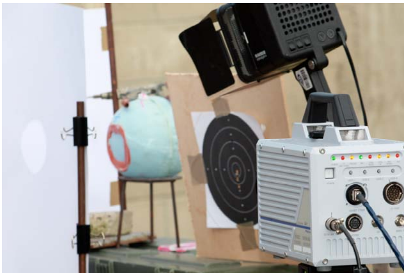
Figure 7.8 The shooting set-up for Model 2. The white paper (left) was positioned in front of the model to record any backscatter. The high-speed camera is in the bottom right of the picture.
