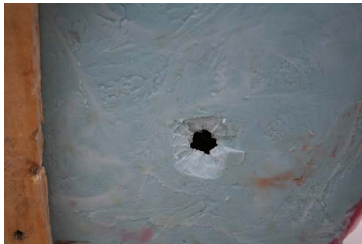
Figure 3.7 The exit wound in model 5. External bevelling was present around the central defect.
