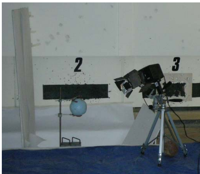
Figure 7.3 The shooting set-up for Model 1. The model was held in place by a clamp stand which was anchored by bricks. The white paper surrounding the model was set-up to catch any backspatter. The high-speed camera is to the right of the picture but is obscured by the light (front).
