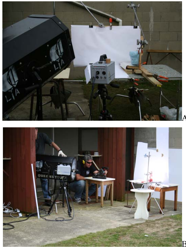
Figure 2.1 Experimental set-up. A: The model (light blue) surrounded by a white paper background with the light (black) and high-speed camera (grey) slightly in front. B: A view of the whole set-up, including the shooter.
