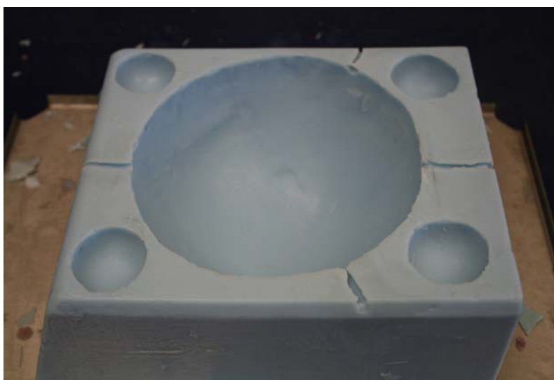
Figure 7.1 The negative mould for creating Spherical model 1. The holes in each corner lined up with those in the positive plugs and therefore acted as orientation points. Run-off channels on each side allowed excess material to escape.
