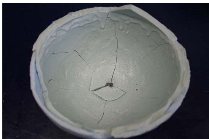
Figure 7.4 The inside view of Model 1A (gelatin removed) showing inward beveling of the bone simulant. Six radiating fractures and four concentric fractures were produced. This fracture pattern and internal beveling was similar to that seen in the three other models.
