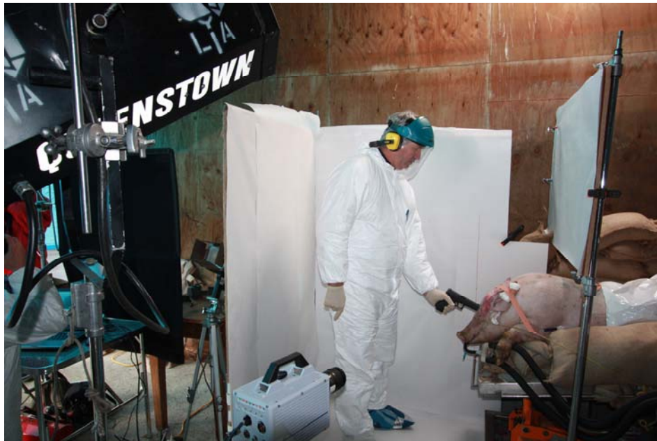
Figure 5.2 The shooting set-up for the contact shots. For the distant shots the shooter stood behind the board which is directly behind him in this figure. A small hole was made in the board for the bullet to pass through.
