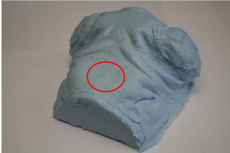
Figure 3.3 The pig head model. The red circle represents the area where the models were shot and where a layer of sponge was present in the blood models. The small slit to the right of this circle was where the eye was in the original pig head used to cast the mould.
