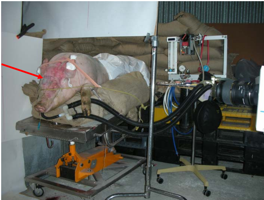
Figure 5.1 The pig positioned on the surgical table, with the anaesthetic and monitoring equipment to the right of the figure. Sandbags were placed below and behind the pig for safety reasons. The arrow indicates the 1 cm x 1 cm grid drawn on the pig's head.
