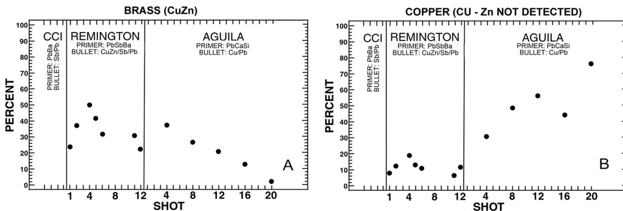
**Fig. 13 A** Graph of percentages of GSR particles with detected brass (CuZn); the Remington bullets were clad with brass. The CuZn-containing particles ranged from 22 to 50% of the population. The Aguila GSR samples showed a gradual decrease in brass-containing particles. **B** Graph of Cu-containing particles (Zn not detected); the Aguila bullets were clad with copper, and Aguila GSR showed a gradual increase in copper-containing GSR with shots
