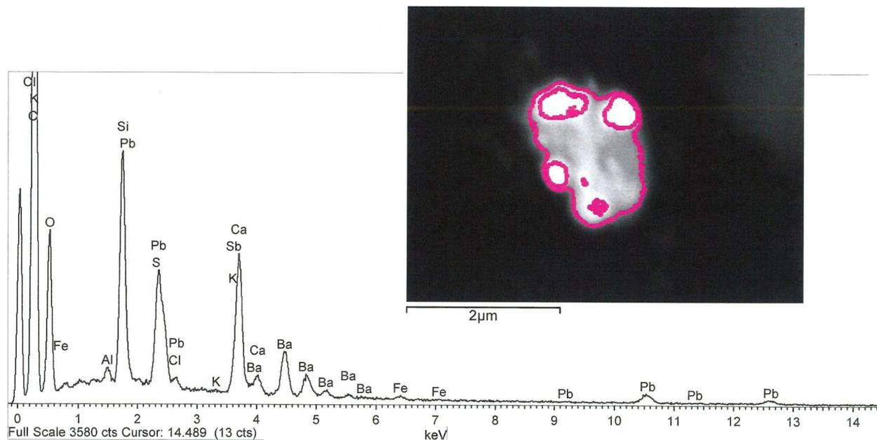
**Fig. 15** A PbBa containing particle from a 9mm pistol discharge with major silicon and calcium peaks; six of these particles appeared similar (BSEI inset), and all seven had similar elemental compositions. Trace Sb was identified in this particle, and the others justified the criminalist's characteristic designation. The other six characteristic GSR particles had a similar morphology. The likely presence of calcium silicide in the origin primer might have influenced the GSR form
