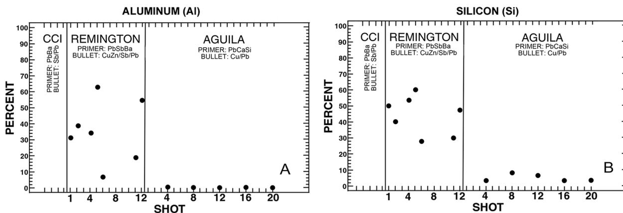
**Fig. 14** **A** Graph of Al-containing breaching GSR; Al was not observed in the Remington GSR from a discharged casing. Al was not observed in any of the samples from the Aguila series. **B** Graph of Si-containing breaching particles; the Remington primer had silica particles as frictionators, which were associated with the breaching GSR. The Aguila had a much smaller amount of silicon despite having calcium silicide as a primer component
