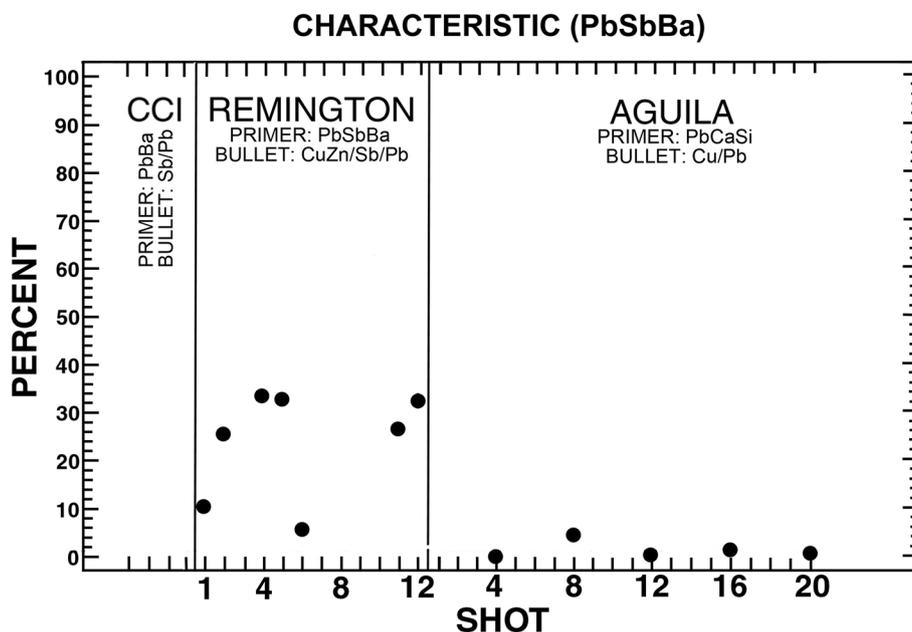
**Fig. 10** Graph of characteristic (PbSbBa) GSR percent composition from the Remington primer discharges to the Aguila; there were small, apparent periodic mobilizations, of residual GSR of characteristic GSR in the Aguila breech samples 8 (6 particles) and 16 (1 particle)
