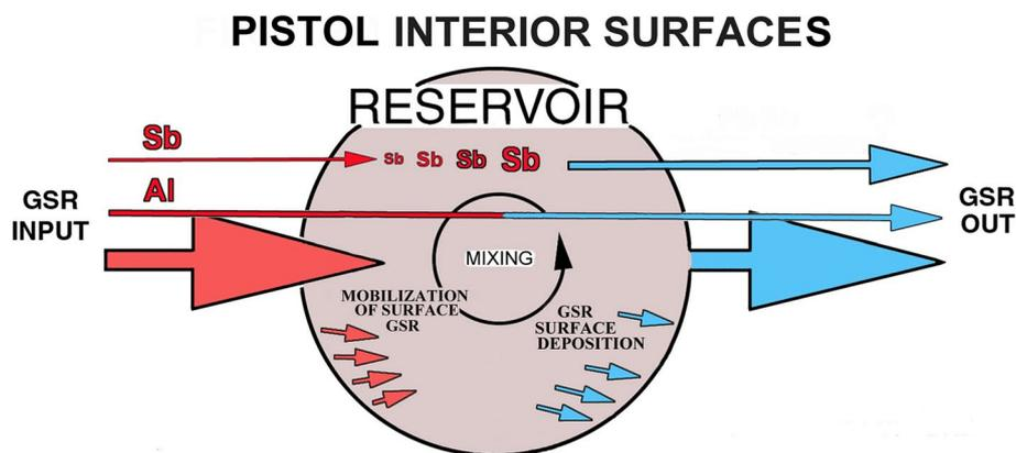
**Fig. 16** The GSR reservoir hypothesis for the creation of pistol breech GSR; the behavior of GSR elements in this proposed reservoir is based on observations of the pistol experiment and may differ in other firearms. In this case, PbSb accumulates on the interior surfaces before being released, likely due to reduction of PbBa concentration within the pistol
