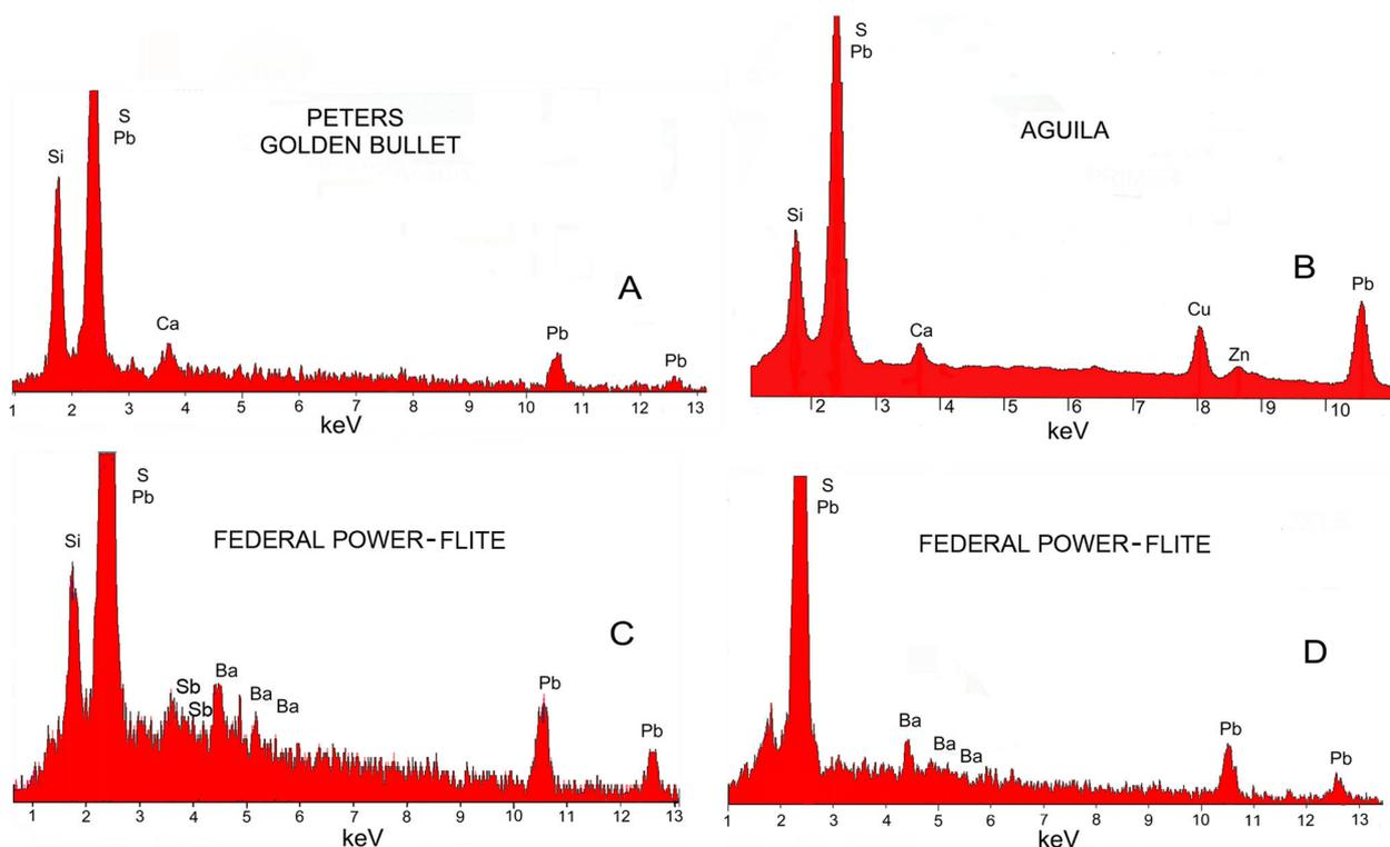
**Fig. 5** **A** Spectrum of Peters Golden Bullet unfired lead/calcium silicide ( $PbCaSi_2$ ) primer. **B** Spectrum of Aguila fired lead/calcium silicide ( $PbCaSi_2$ ) primer; the CuZn is from the casing. **C** Spectrum of Federal Power-Flite unfired PbSbBa primer. **D** Spectrum of Federal Power-Flite unfired PbBa primer
