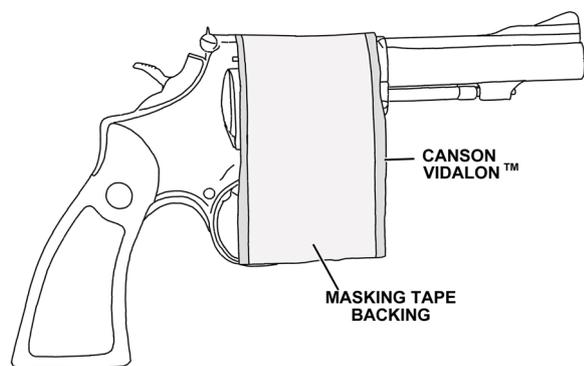
**Fig. 1** The Smith and Wesson Model 18 revolver with the attached vellum backed by masking tape draped over its side to intercept cylinder gap GSR, minimizing retrograde muzzle GSR contamination. The exit port of the Ruger MKII pistol was similarly draped for breach GSR collection
