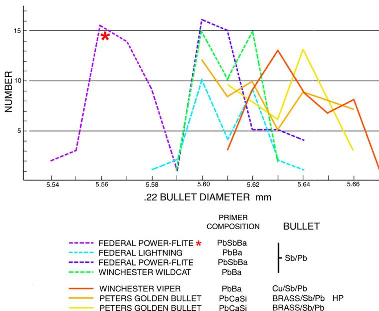
**Fig. 3** Graph of the diameters of seven brands of .22 caliber bullets; fifty bullets were measured from each brand. The asterisked Federal Power-Flite bullet diameters are smaller than the other .22 caliber bullets
