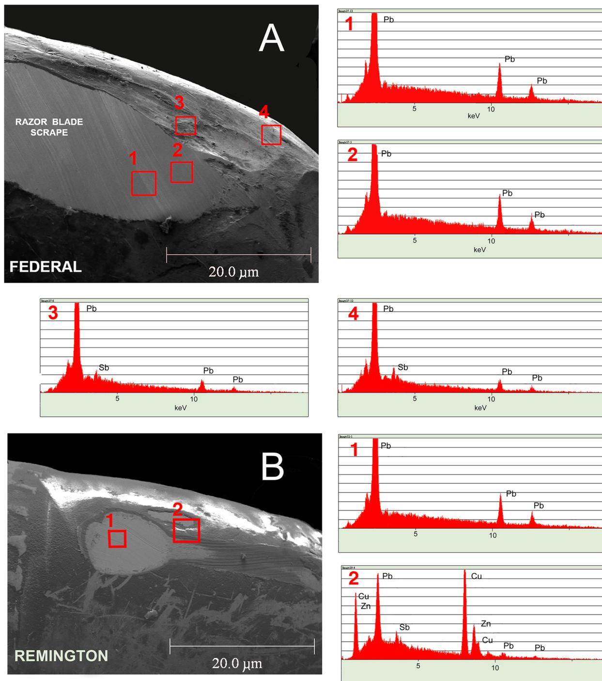
**Fig. 4** Antimony surface layers on two .22 caliber bullets. **A** The surface of a Federal Power-Flite bullet that had been scraped by a razor blade; Sb was not detected in areas of EDS samples 1 and 2 from the razor scrape area but was detected in areas of the unscraped bullet (EDS areas 3 and 4). **B** The scraped surface of a Remington Golden Bullet upon which beam rastering (EDS area 1) did not detect Sb; Sb was detected in EDS area 2 on the unscraped surface
