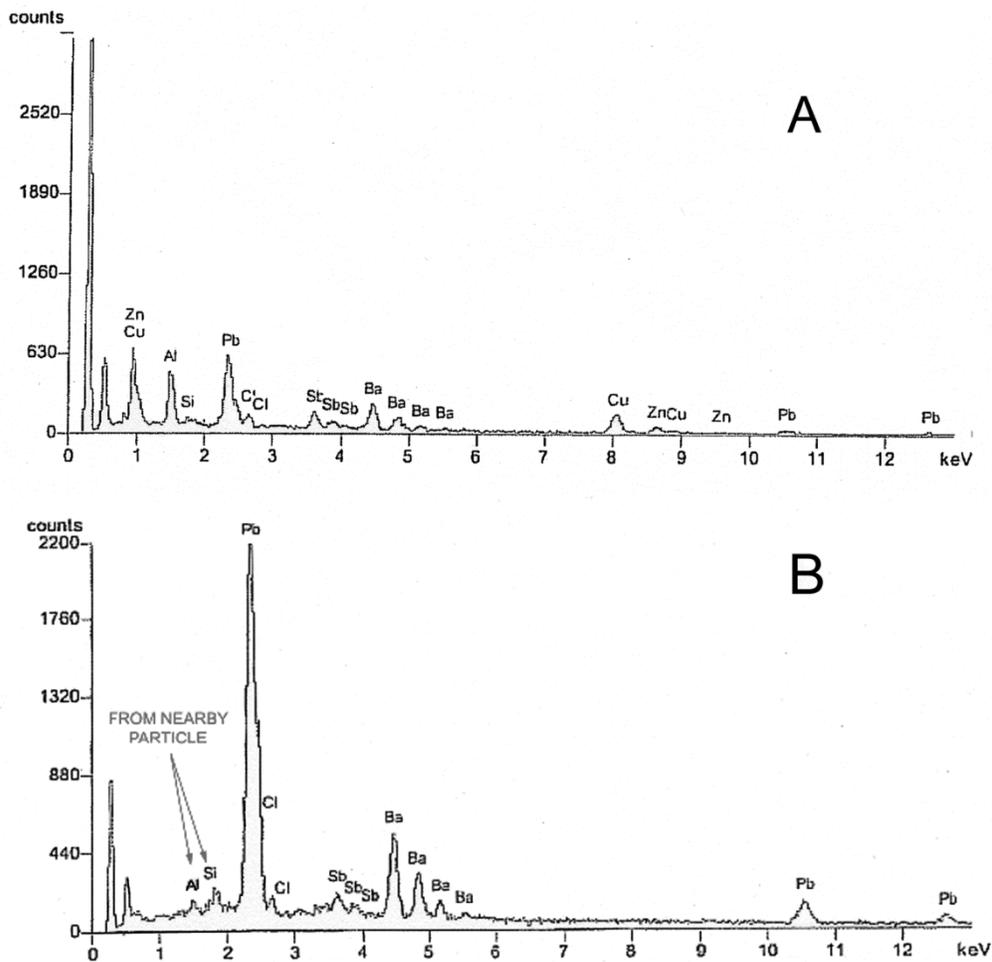
Figure 1. Example spectra from the Lyons case. A. A typical example spectrum of a characteristic GSR particle from the hand sampler of Corey Lyons that also contains aluminum and copper; detectable amounts of zinc were found in a number of these particles, but were not considered in the statistical analysis. B. A typical example spectrum of a characteristic GSR particle from objects associated with Lyons and hypothesized to have been handled by Lyons.
