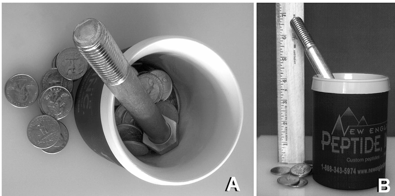
**Figure 1.** A: Image taken with the Pixera 600CL camera through the Computar MLH-10X macro zoom. B: Image taken from the side of the bolt in the cup. A ruler documents the difference in elevation from the end of the bolt to the quarters on the table. Details on the US quarters as well as texture at the end of the bolt are seen despite a 200 mm (7 7/8 inches) difference in elevation. Image depth of field/field width equals approximately 1.
