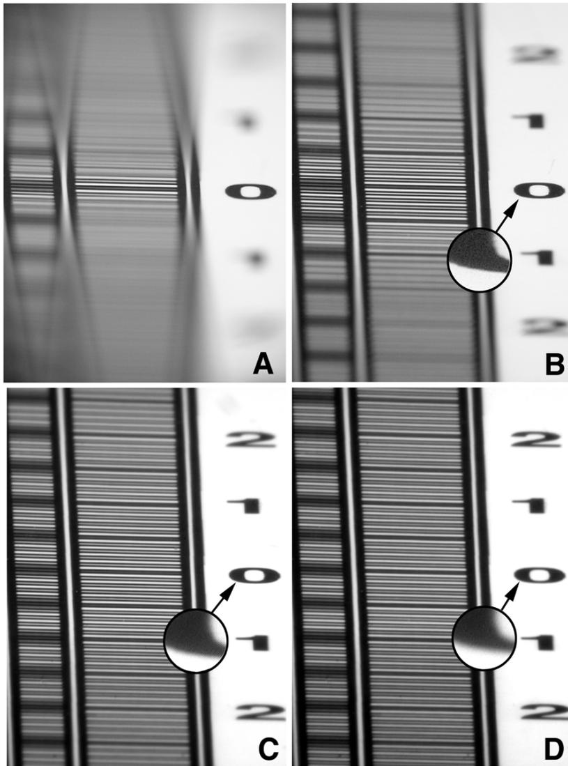
**Figure 3.** Images from the Pixera 600CL tests at the field width of 20 mm. A: The depth of field target at  $f$  5.6. B: The target image at the same position at  $f$  32. C: The target image at one f-stop greater than  $f$  32 (2.8 sec exposure at ISO 200 setting for the camera, 10 frames averaged). D: The target image at two f-stops greater than  $f$  32 (5.2 sec exposure at ISO 200 setting for the camera, 10 frames averaged).
